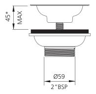
\*Suitable for granite, composite and vitreous china sinks with a material thickness up to 45mm.
