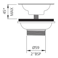
\*Suitable for granite, composite and vitreous china sinks with a material thickness up to 45mm.
